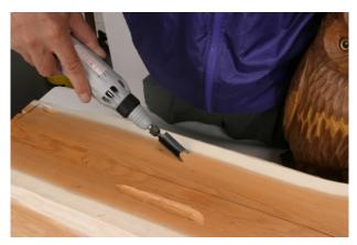
Powerful motor is built in, and the machine can be used just by plugging it in your wall power receptacle. Its blade reciprocates at super-high speed (12,000 times per minute) and in tiny travel (1mm back and forth), and it can carve hard wood and others with one third of force needed in carving by hand.
